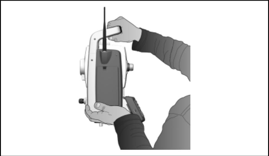
Figure 4.42 Correct way to lift the instrument
